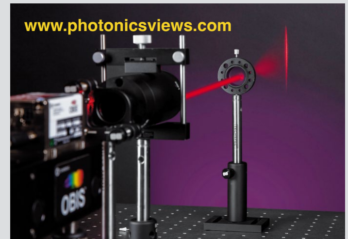
Laser line generation setup with a cylinder lens
